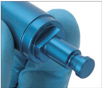
The counter part of the Hudson coupling at the perforator drill has to be inserted aligned with the notch of the other part.
